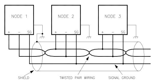
Figure 2-7. Preferred Multipoint Wiring Using Shielded Twisted-pair Cable with a Separate Signal Ground Wire
