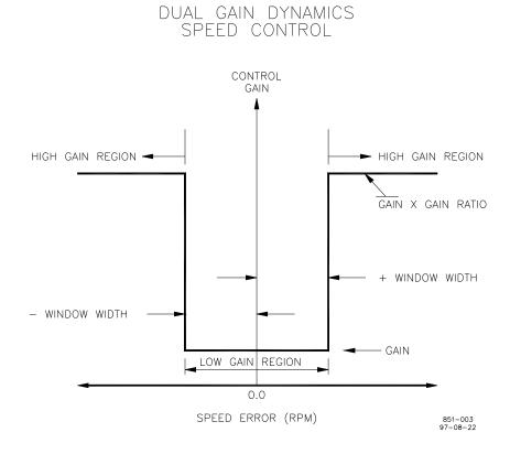
Figure 3-14. Control Gain as a Function of Speed Error
