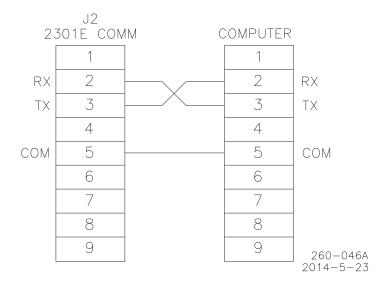
Figure 3-1. Null Modem Cable
