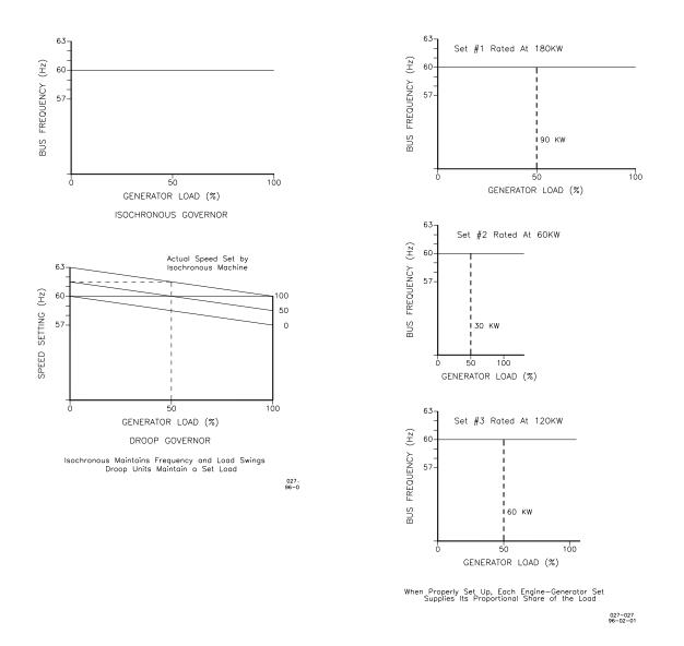
Figure 4-9. Droop/Isochronous Load Sharing
