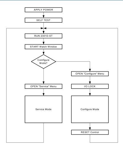
Figure 4-1. Basic Operational Architecture
