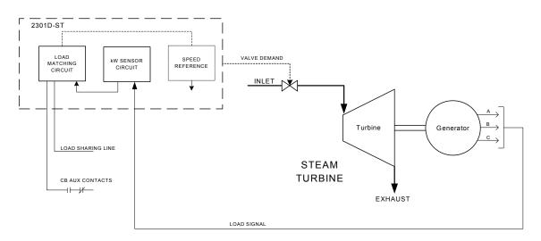
Figure 4-6. Paralleling System
