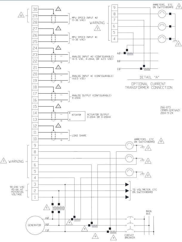
Figure 2-2a. 2301E-ST Plant Wiring Diagram (sheet 1)
