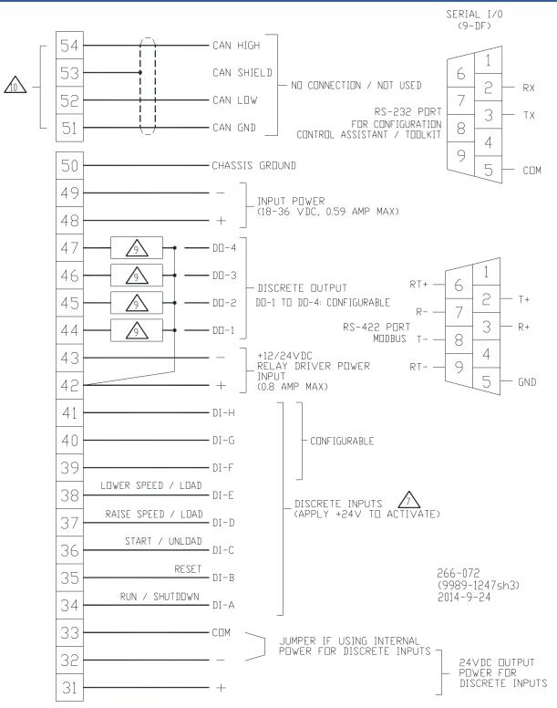
Figure 2-2b. 2301E-ST Plant Wiring Diagram (sheet 2)
