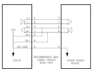
Figure 2-5. Typical RS-422 Communications Connections
