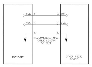
Figure 2-4. RS-232 Pin assignments for Serial Communication Cable
