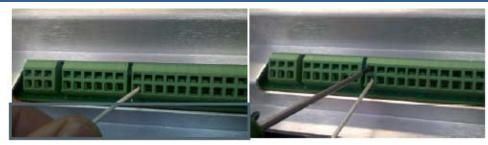
Figure 2-3. Installation of Wiring into Terminal
